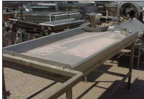
It is important at this step to reject any leaves with evident injuries, cuts, or lesions in order to avoid contamination of the product downstream. Tips, tails, and spines are usually cut off the leaves by hand at this stage, so again the layout is such that would accommodate enough people to perform these duties. Typically 6 to 8 people can process 1000 Kg of leaves through this step.
